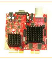
**Figure 4** I The Gizmo board leverages an AMD Embedded G-Series APU to provide 52.8 GFLOPS of performance under 10 W.
