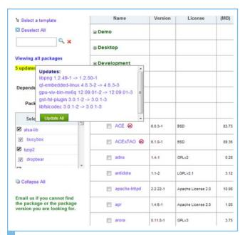
**Figure 1** | A LinuxLink update engine informs platform engineers when updated versions of open source software packages are available for download.
