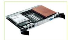
Figure 2 | Kontron's CP6005-SA family uses 4th generation Intel Core i7 processors.
