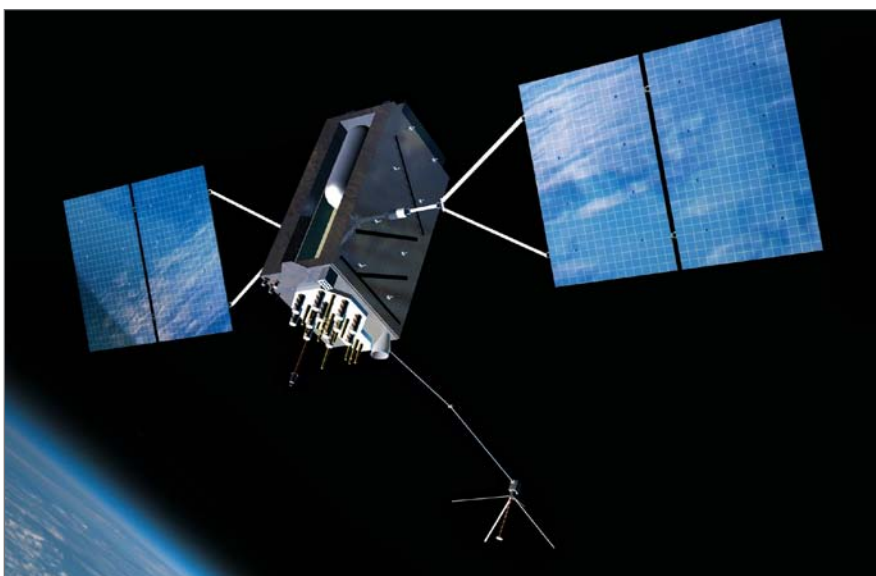
Figure 1 | The GPS III satellite from Lockheed Martin makes use of radiation-hardened electronics for its payload and control systems. Photo courtesy of Northrop Grumman, whose Astro Aerospace business unit supplies self-deploying, monopole JIB antennas for the satellite.
