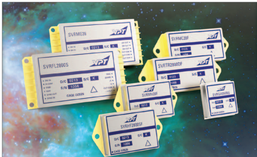
Figure 2 | VPT's SVR series products are qualified to 100 krad(Si) and 85 MeV-cm2/mg SEE performance with displacement damage performance.
