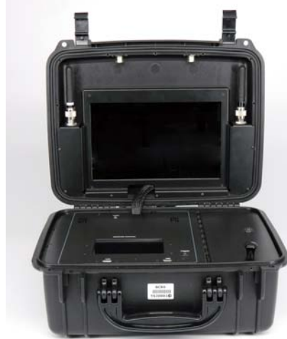
Figure 6 | The BCRx is a diversity receiver/monitor integrated into a ruggedized, portable IP66-rated briefcase. Photo courtesy of Integrated Microwave Technologies.
