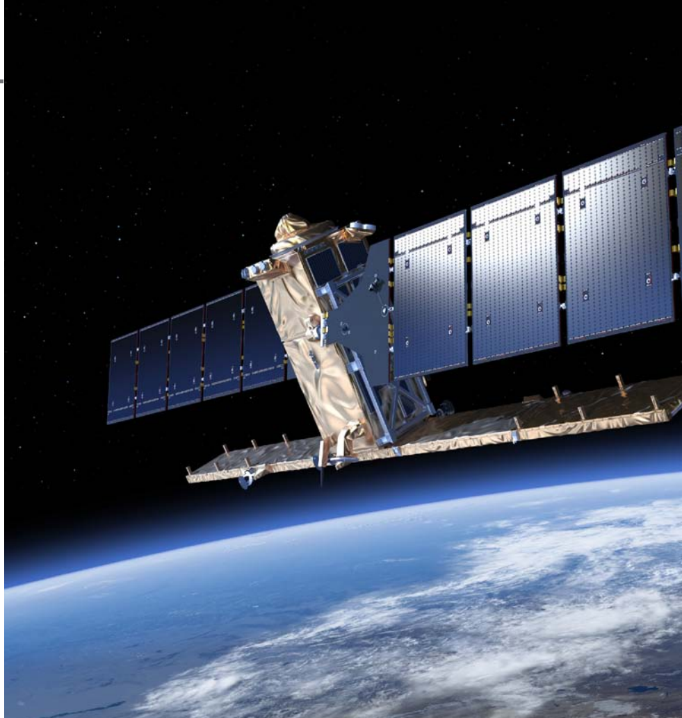
Sentinel-1, the first of the European Space Agency's Copernicus satellites, will monitor aspects of Earth's environment, from mapping sea ice to detecting and tracking oil spills to monitoring movement in land surfaces. Photo courtesy of the European Space Agency (ESA)/ATG medialab.
